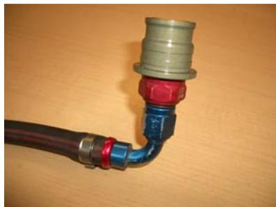
3. Slide the 2x 17.5mm Oeteka Clips (A082L6227F ) over the hose and press the T Piece (ALS3L0070F) into the opposite end.
