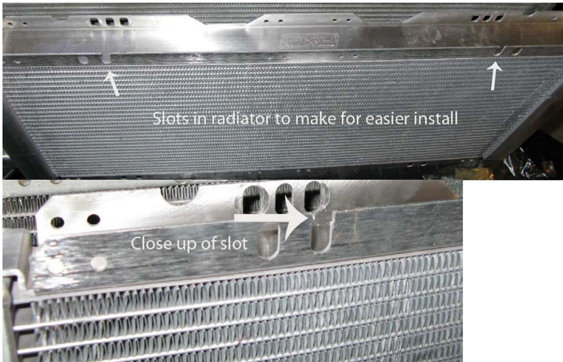
9. Slide new radiator into place and bolt back in place (Note: Leave bolts loose till you have all bolts in place before tightening down.)
