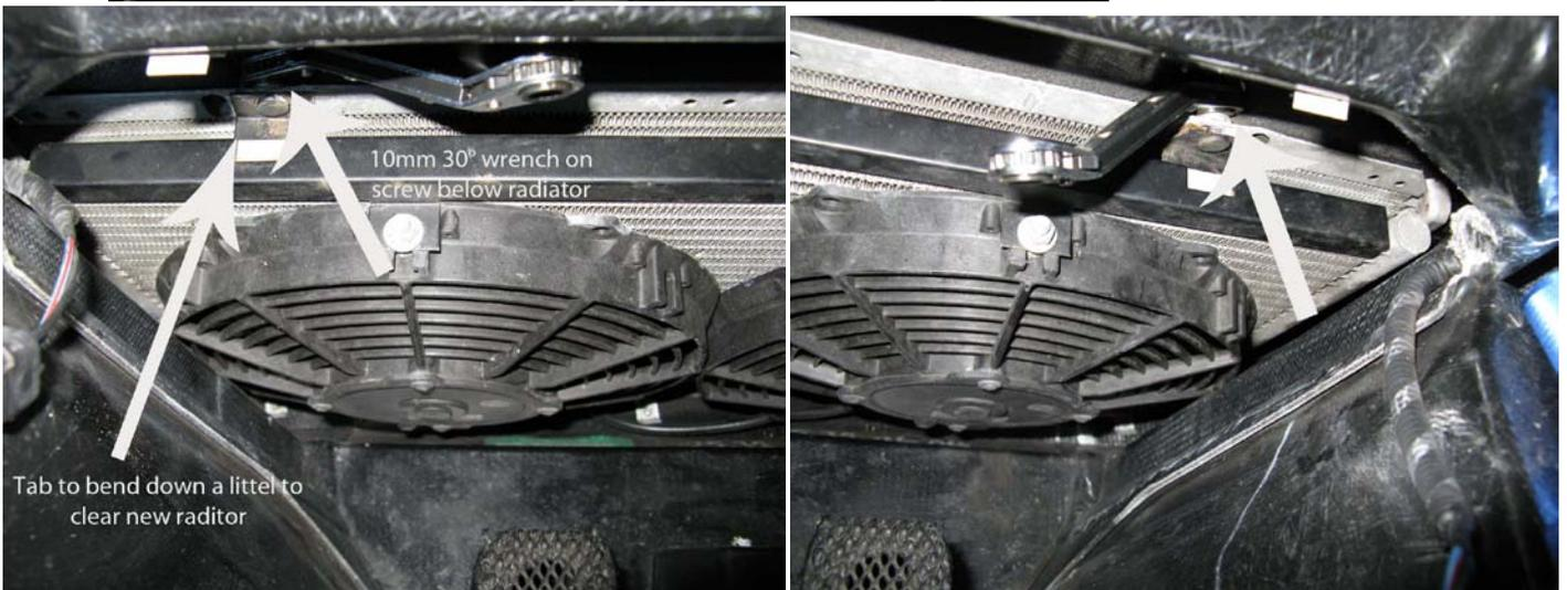
4. Scrape the foam on the sides of the radiator with a long flathead screwdriver to release it. (be careful not to hit the condenser below it)
