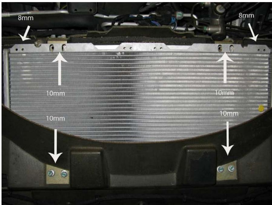
3. Remove the bolts on the underside holding the fan to the radiator.
